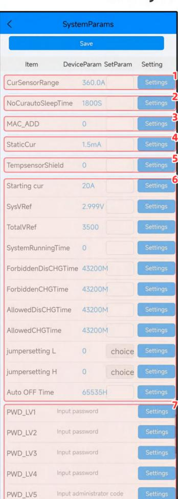
1 If the current detected by the protection board is not accurate with the actual value, you can use this value. Each time you increase or decrease it by 10, the current will become larger and smaller accordingly. Repeatedly modify the value to check the current until the displayed current is equal to the actual current. You need to Use a high-precision multimeter to measure, and the error range is within 5%.
