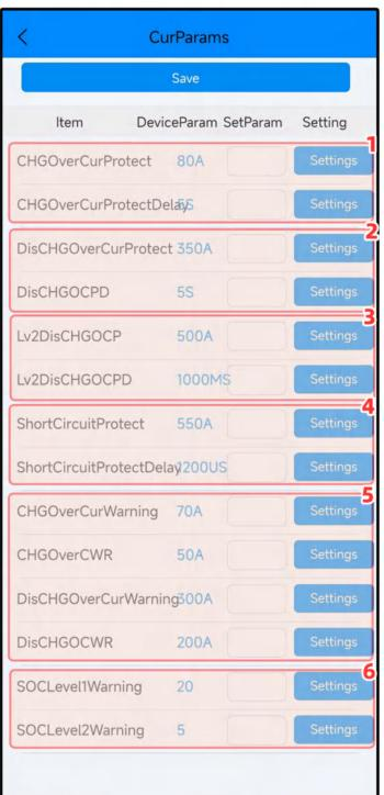
1 Indicates that the charging current exceeds 50A and lasts for more than 5 seconds, and the charging overcurrent protection will be triggered.
